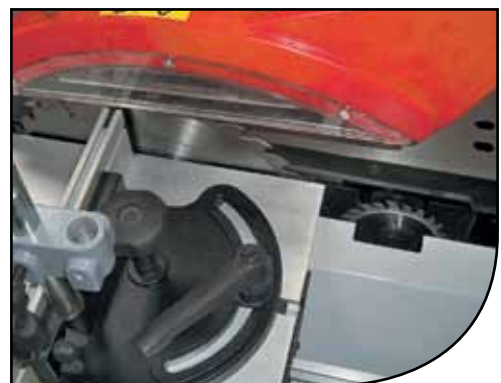
Chariot ras de lame 2000mm, lame ø 315, inciseur ø 100mm Sliding table's guide 2000 mm, blade ø 315 mm, scoring blade ø 100 mm
